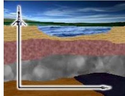
Hydraulic fracturing (or fracking) is a technique that was first used at the end of the 1940s. It injects large amounts of water, under high pressure, combined with chemicals and sand, into the shale formation. The quantity, characteristics, and toxicity of the chemicals are disputed. This fragments underground rock, creating pathways for otherwise trapped natural gas (and oil) to find a route and flow through to the well.<sup>29</sup>
