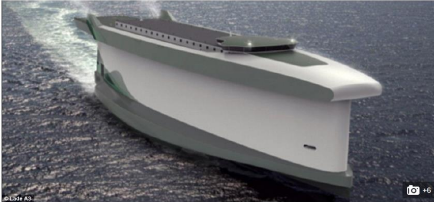
The Vindskip (pictured), designed by Lade AS, uses a hull designed to act as a so-called airfoil, or giant sail. The makers of the wind-powered hybrid merchant ship said that while engines are still needed, their design could achieve fuel savings of 60% while reducing emissions by 80%.
