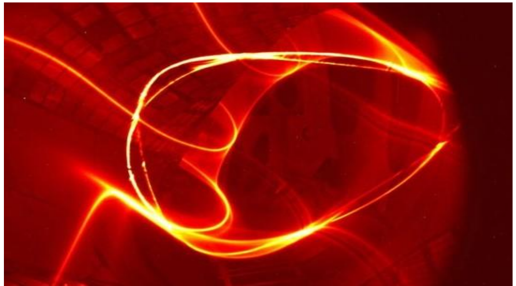
Figure 2: Magnetic field surface in the Wendelstein 7-X stellarator
